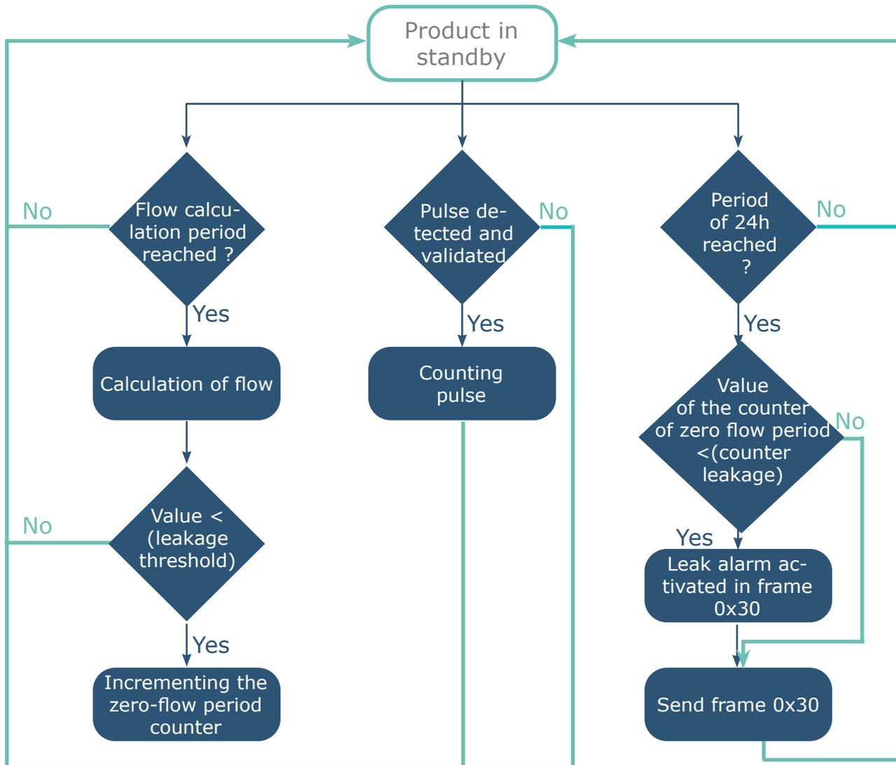
The flow rate corresponds to the number of pulses of the flow calculation period divided by the same period. It is expressed in pulses / hour.
