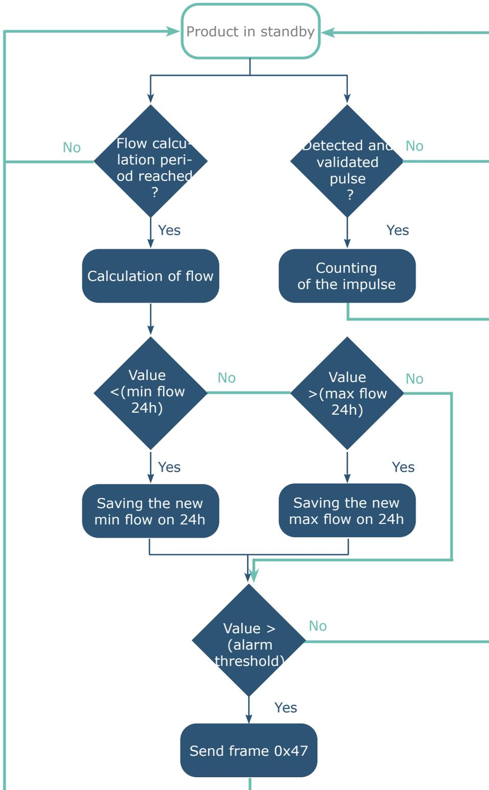
The flow rate corresponds to the number of pulses of the flow calculation period divided by the same period. It is expressed in pulses / hour.
