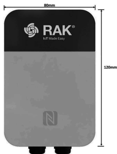
Figure 1: RAK2560 WisNode Sensor Hub dimensions
