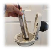
Measure and note the distance **B** from measuring point to water surface.
