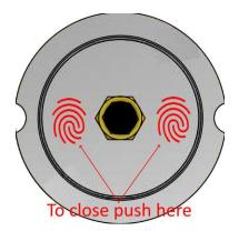
To close the unit, push with two fingers against the top of the housing/piston until it stops. Be sure that that the piston is completely inserted. Keep dry before opening and closing. To close the ADT1 Box you just squeeze the screws together and make a quarter turn.
