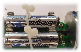
Insert 3 high-quality lithium AA batteries (Energizer Ultimate Lithium / L91) into the battery holders. Always replace all three batteries simultaneously with identical and new ones. Makes sure you insert the batteries the right way as shown in the picture. The device operates until the voltage drops to 3.5V
