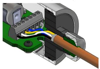
Connect the black wire to the +3.5V supply voltage and the white wire to the GND pin.
