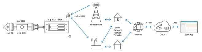
The LoRaWAN® module, which can be configured on a country-specific basis, establishes a connection with a LoRaWAN® <u>Gateway</u> and makes it possible to send the measurements to a <u>LoRa network server</u>. The LoRaWAN provider can be selected freely. The easiest and most convenient way to access the collected data at the end of the transmission chain is via <u>KOLIBRI Cloud</u> from <u>KELLER</u>.
