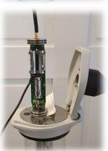
As the inner part of the ADT1 is pulled out, the position of the level probe changes by 16.5 cm, i.e. the length of the inner part.
